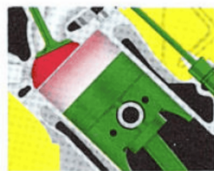
"hi-swirl" combustion chamber
