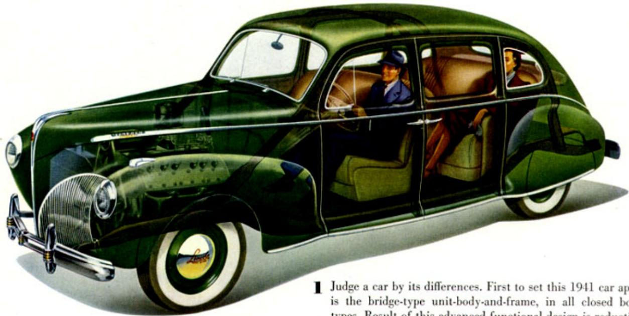
**1** Judge a car by its differences. First to set this 1941 car apart is the bridge-type unit-body-and-frame, in all closed body types. Result of this advanced functional design is reduction in weight, improved economy of operation, great strength.
