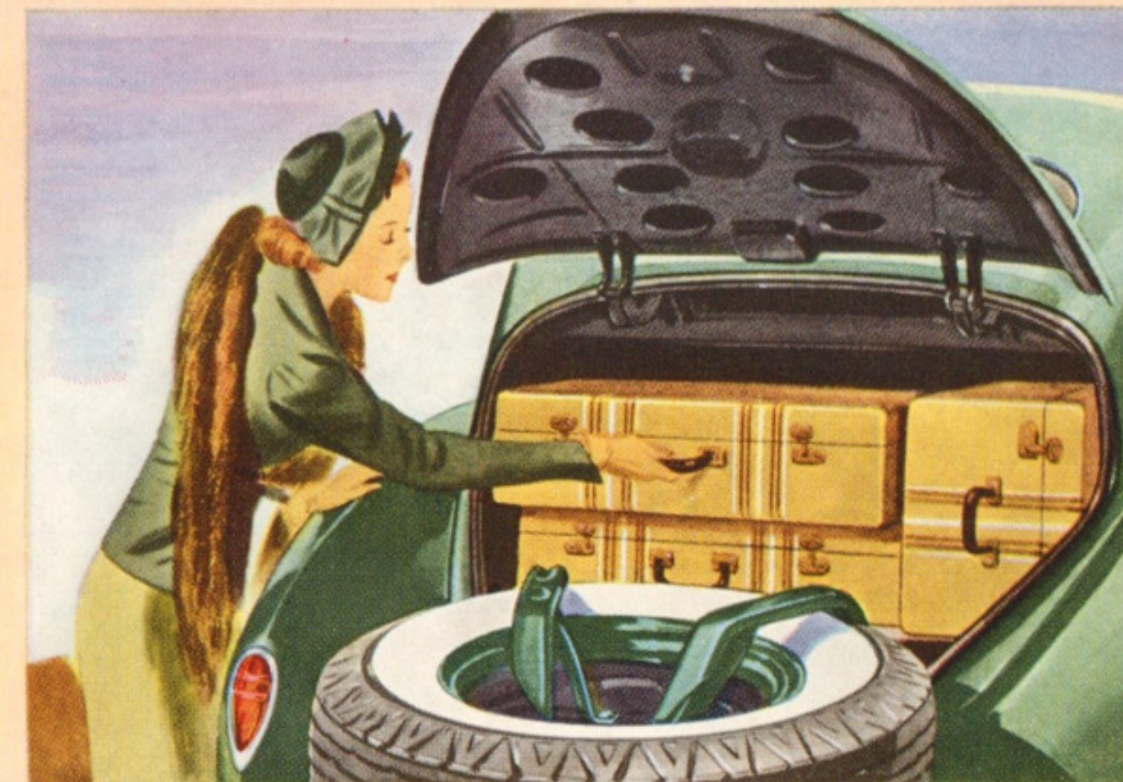
SPACIOUS LUGGAGE COMPARTMENT —the large luggage compartment in the rear deck (automatically lighted) is lined, and is dust-proof and water-proof. The spare tire and wheel, also carried here, swing outward easily.
