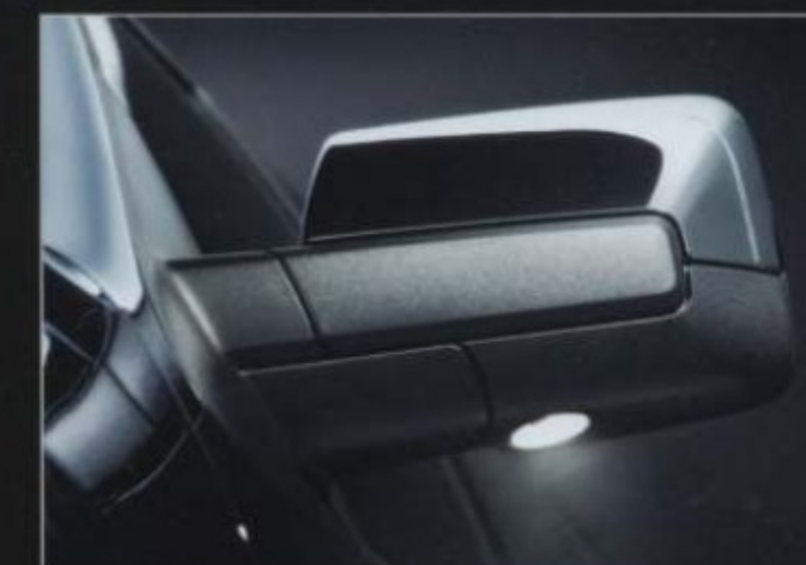
Power-folding heated sideview mirrors feature security approach lamps that activate when your key fob is pressed.
