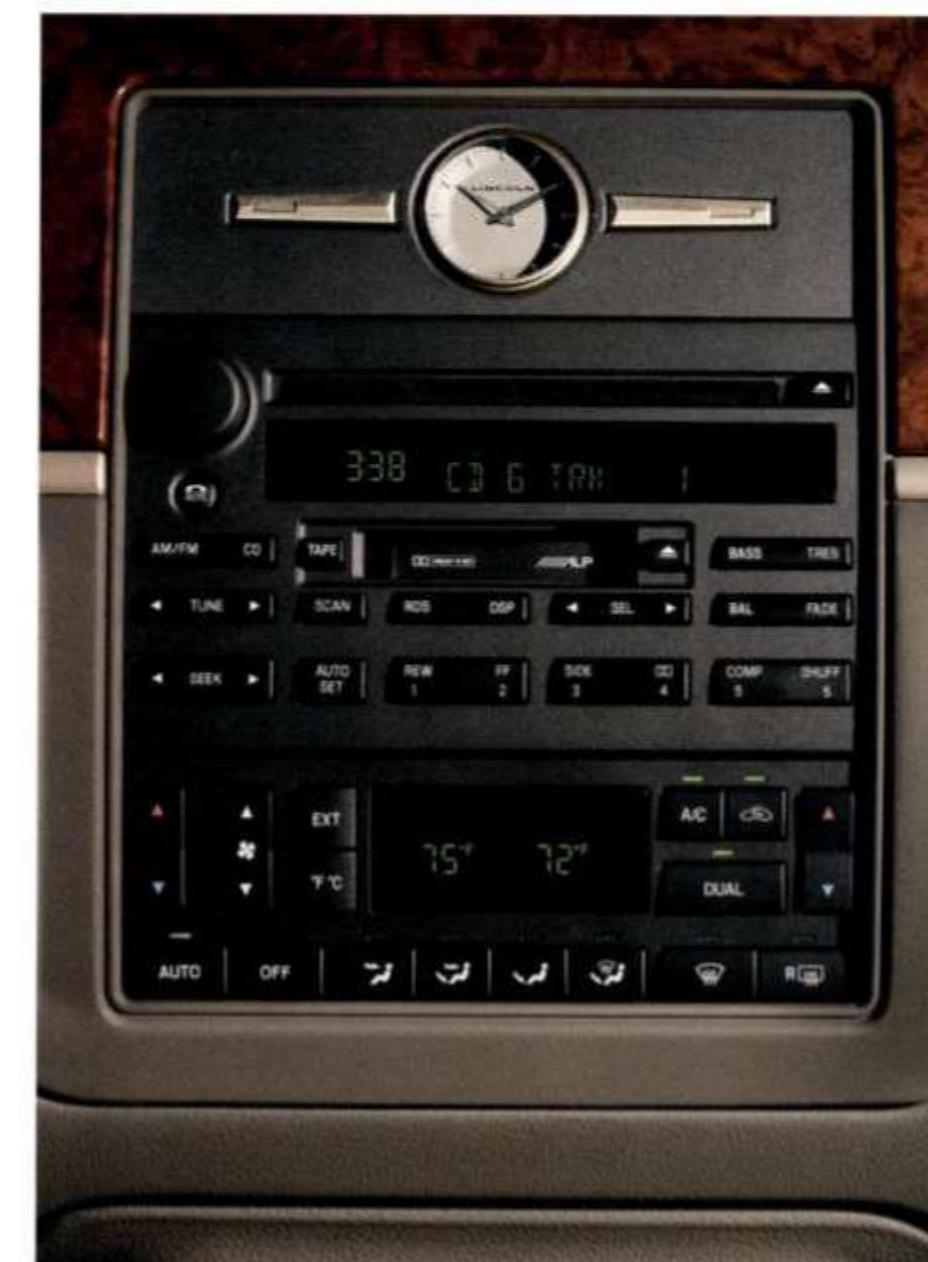
The Dual-Zone Electronic Automatic Temperature and audio controls are conveniently located centrally between the driver and front passenger to ensure equal accessibility and comfort.
