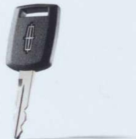
This is no ordinary key. This electronically coded ignition key is the hub of the Lincoln LS Securilock<sup>®</sup> passive anti-theft system. It prevents ignition bypass by allowing only the correctly coded key to start the vehicle. The security system is also armed once the key is removed from the ignition and disarmed only with the correctly coded key.
