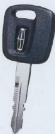
This is no ordinary key. This electronically coded ignition key is the hub of the Lincoln LS SecuriLock™ passive anti-theft system. It prevents ignition bypass by allowing only the correctly coded key to start the vehicle. The security system is also armed once the key is removed from the ignition and disarmed only with the correctly coded key.
