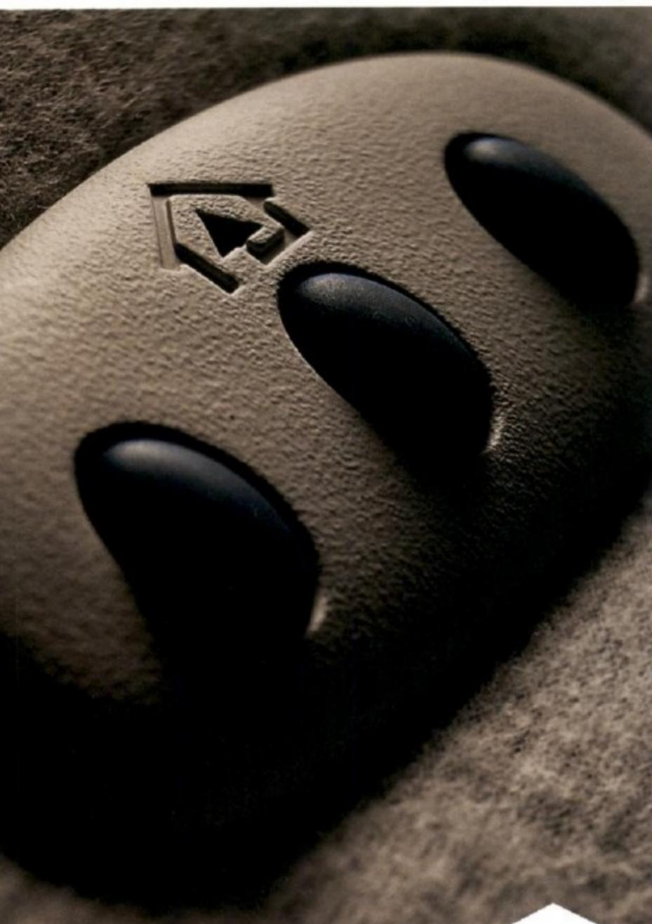
Located in the driver's visor, the standard **HomeLink**<sup>®</sup> allows up to three remote devices—your garage door opener or patio and driveway lights, for example—to be activated from inside Continental. This will eliminate the frustration of having to juggle old-fashioned hand-held remotes while trying to park or depart.
