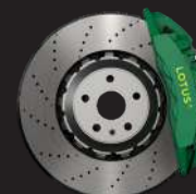
6 PISTON - FRONT GREEN CALIPERS LIGHTWEIGHT BRAKE DISCS (NO COST OPTION)
