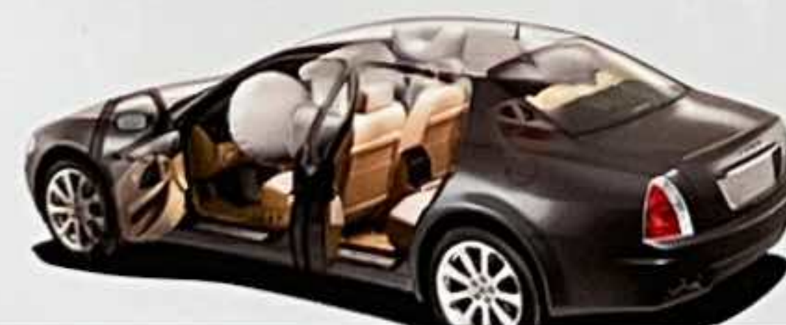
Airbag layout with 6 standard airbags
