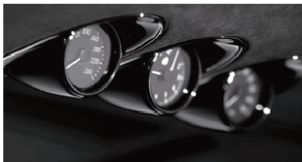
The three beautifully finished duplicate instruments keep the rear passengers informed about the car's speed, the time and the outside temperature. Their housing and support are finished in black piano lacquer in the Maybach 62 S
