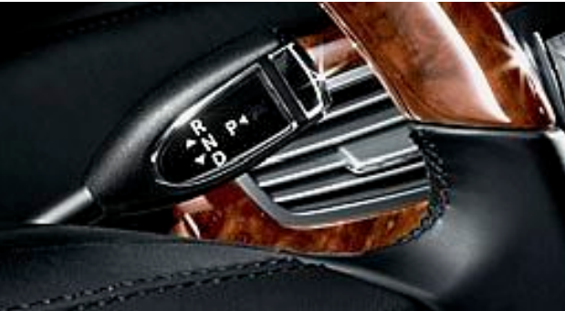
DIRECT SELECT Briefly moving the steering-column selector lever is all it takes to select the driving mode
