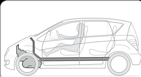
The sandwich design ensures that the A-Class is big on safety too. The seating position is also slightly higher than in a conventional saloon
