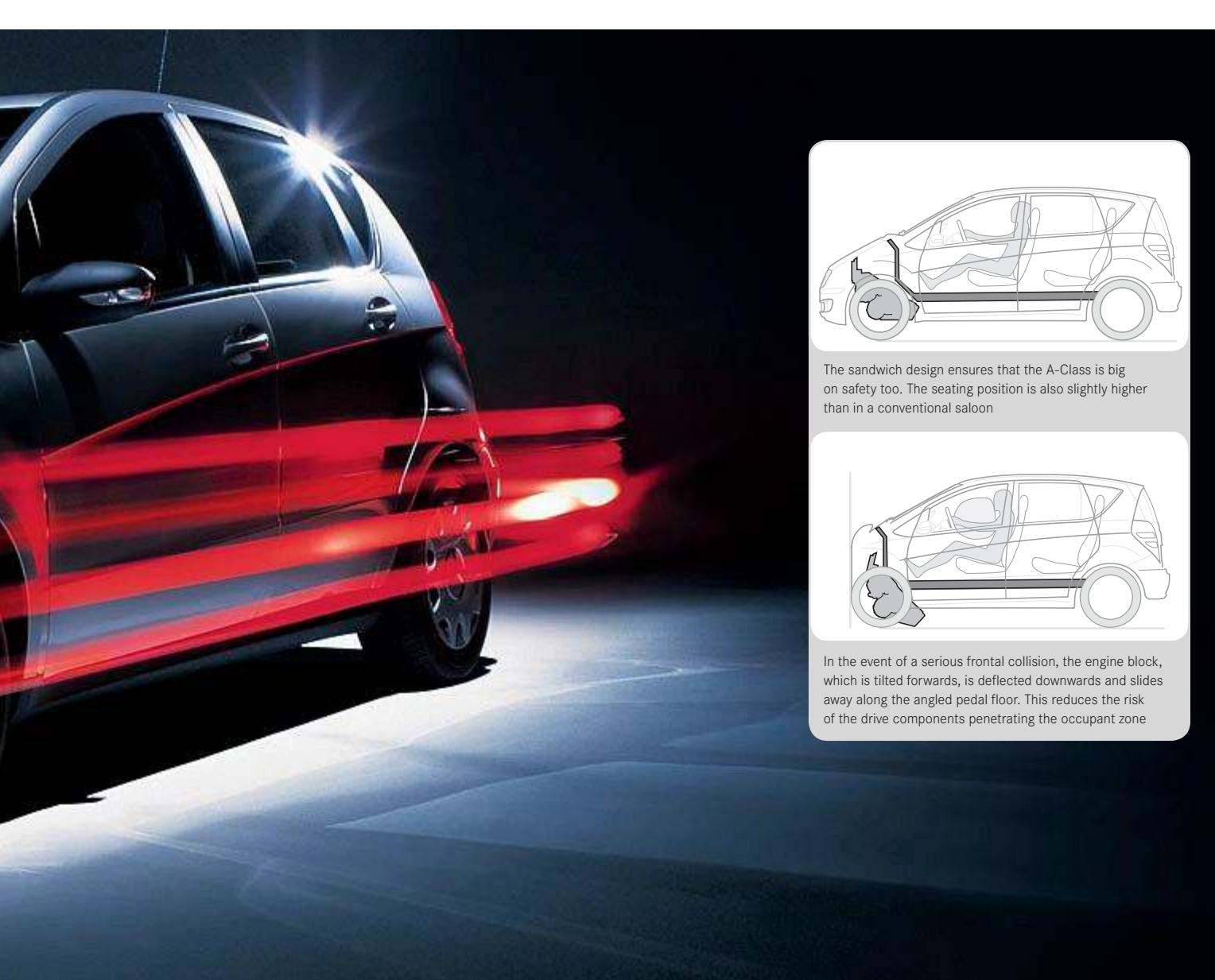
*You can tell from its shape that the A-Class is unlike any other car. It is based on a unique principle, the sandwich design. An intelligent form of crumple zone, this principle also has benefits in a side impact, since the seating position is somewhat higher than in a conventional saloon*
