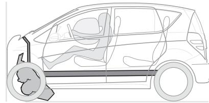
In the event of a serious frontal collision, the engine block, which is tilted forwards, is deflected downwards and slides away along the angled pedal floor. This reduces the risk of the drive components penetrating the occupant zone
