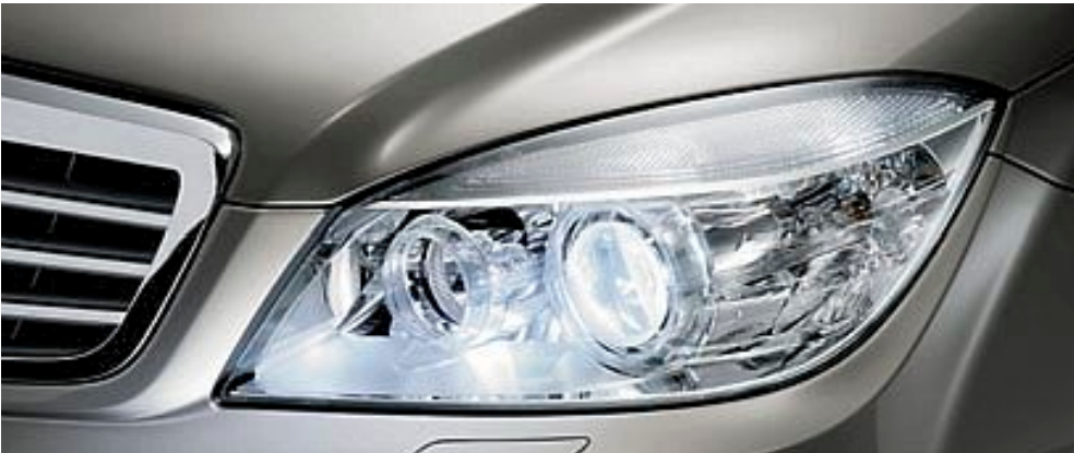
Intelligent Light System with bi-xenon headlamps
