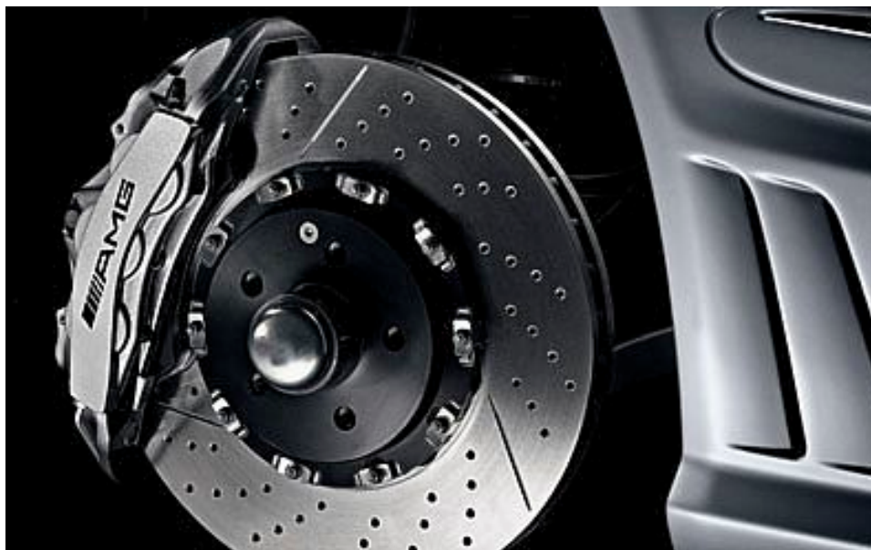
AMG braking system with composite brake discs
