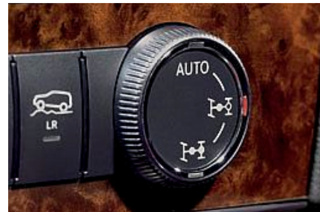
Adjust the differential locks with a mere flick of the wrist
