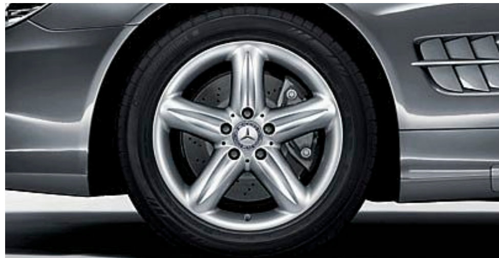
17-inch 5-spoke light-alloy wheels (standard on SL 280)
