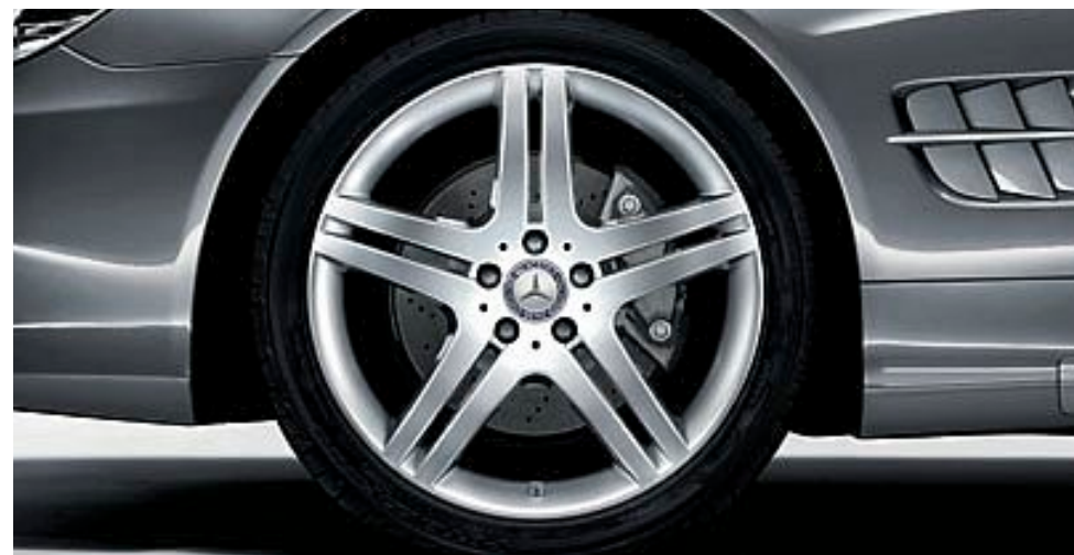
19-inch 5-twin-spoke light-alloy wheels (standard with sports package, optional extra on SL 600)
