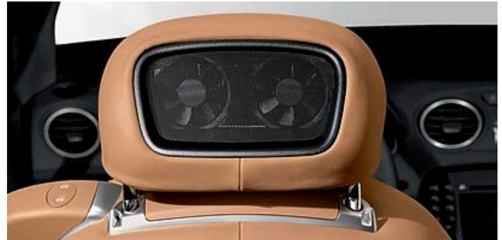
Head restraint with AIRSCARF
