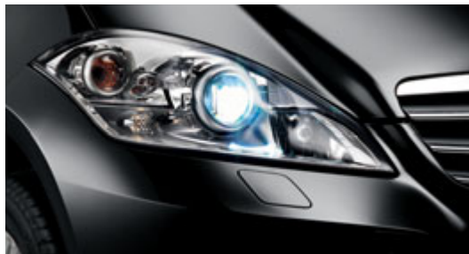
Bi-xenon headlamps / cornering light function for optimum visibility
