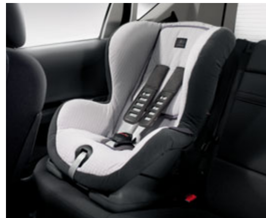
ISOFIX child seat attachment points in the rear with TopTether provide the best possible level of protection for your child, allowing a rigid connection between child seat and vehicle body
