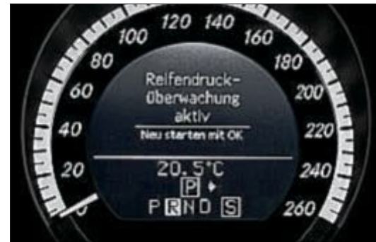
Tyre pressure loss warning system
