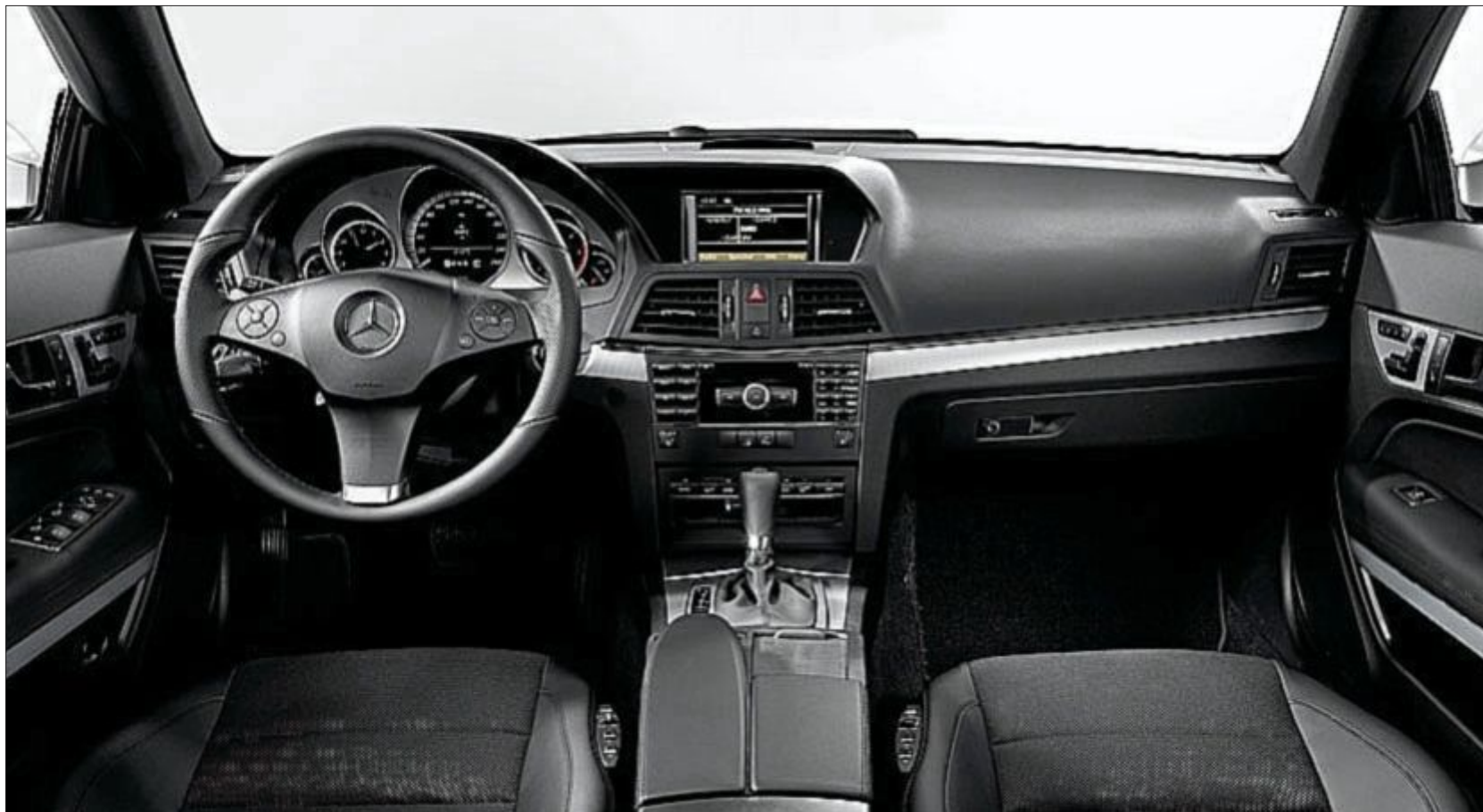
The automatic climate control THERMATIC allows individual temperatures to be set in two vehicle zones
