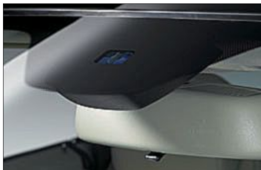
Rain sensor and light sensor for Headlamp Assist
