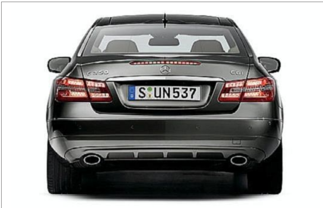
The particularly fast LED tail lights and the adaptive brake lights are an important boost for perceptive safety
