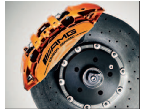
AMG ceramic high-performance composite brake system
