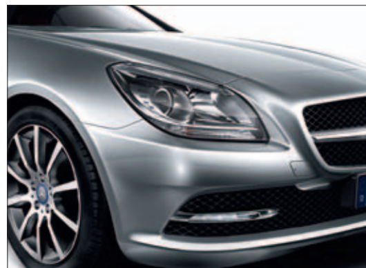
Clear-lens headlamps and LED daytime running lights
