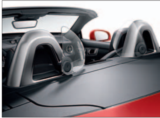
Airguide wind deflector, comprising twin Plexiglas® panels
