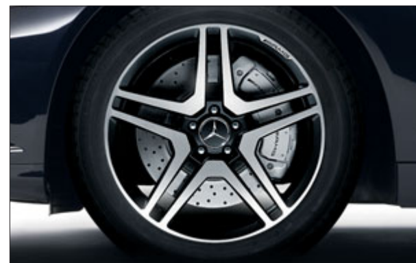
5-twin-spoke AMG forged wheels with 255/35 R 20 front and 275/35 R 20 rear tyres
