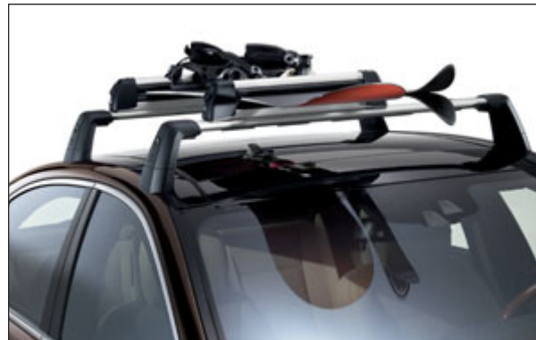
The practical New Alustyle “Comfort” ski and snowboard rack can carry up to six pairs of skis or four snowboards
