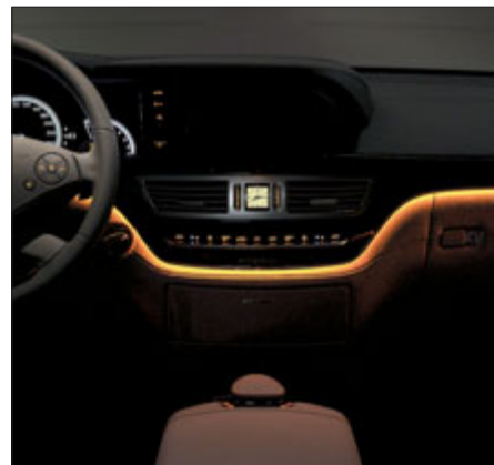
The ambient lighting is a narrow band of LEDs that can light up in three colours
