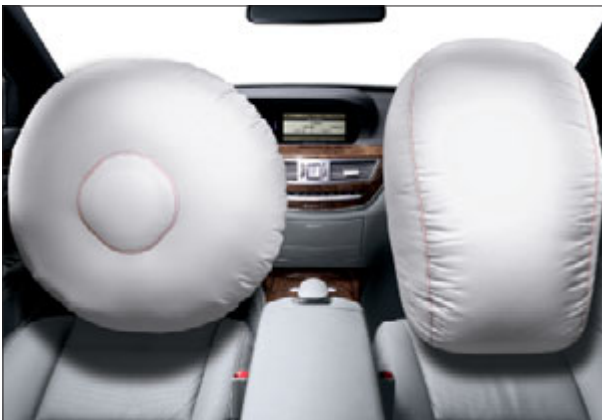
A total of nine airbags can protect you and other car occupants in the event of an accident
