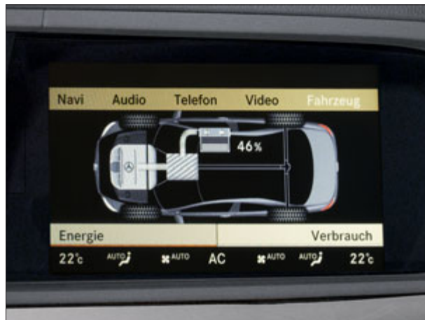
Energy flow display in the S 400 HYBRID model
