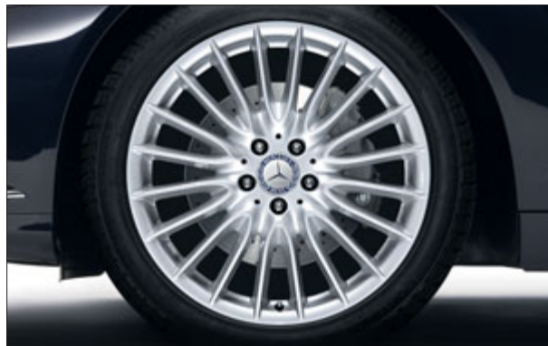
Multi-spoke light-alloy wheels with 255/40 R 19 front and 275/40 R 19 rear tyres (optional extra)
