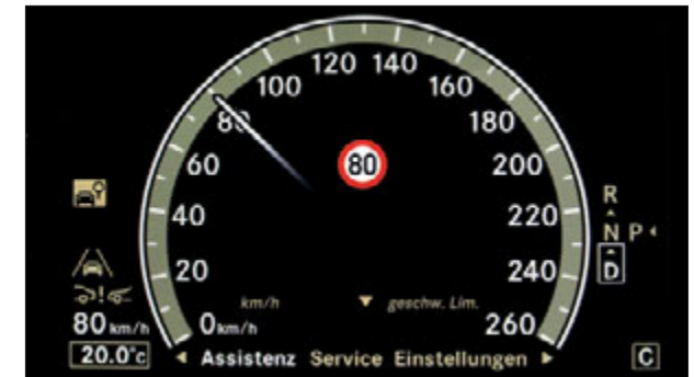
Speed Limit Assist display in the instrument cluster
