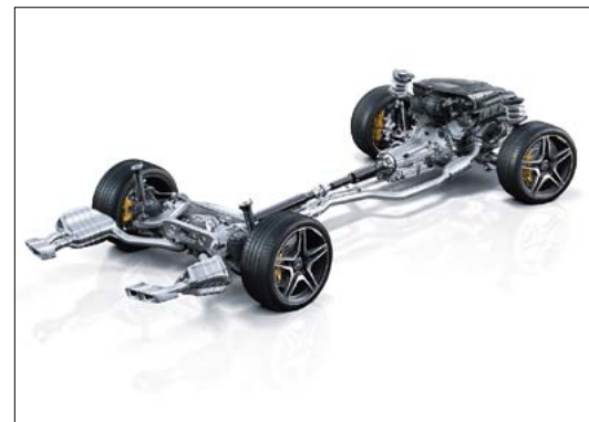
The AMG Ride Control sports suspension with wider front axle offers improved lateral dynamics
