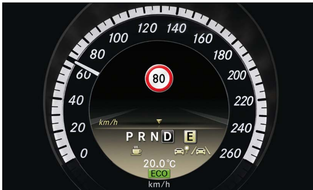
Speed Limit Assist Plus also indicates temporary speed limits
