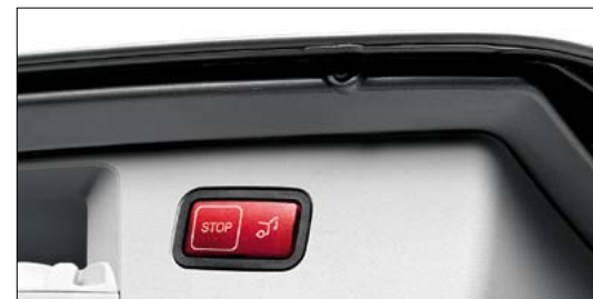
The Easy-Pack automatic powered tailgate opens and closes at the touch of a button and can also be stopped part way
