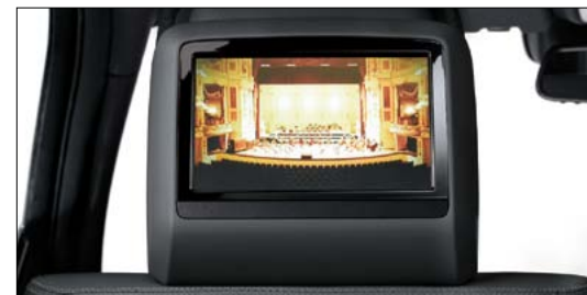
The two displays for the rear seat entertainment system are integrated in the front-seat head restraints
