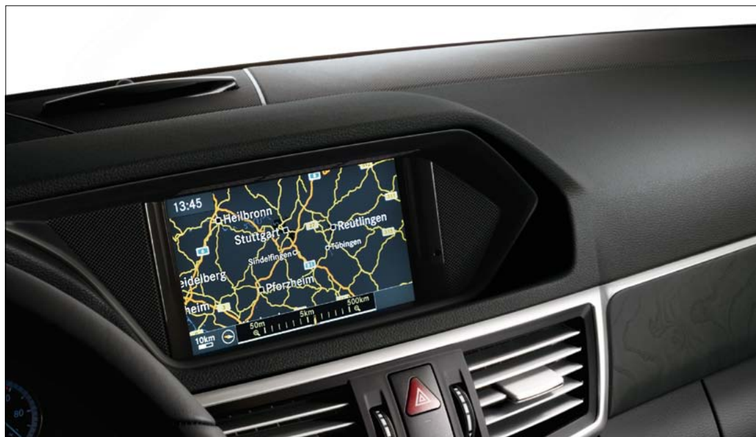
COMAND Online combines telephone, audio and navigation functions and includes Linguatronic voice control
