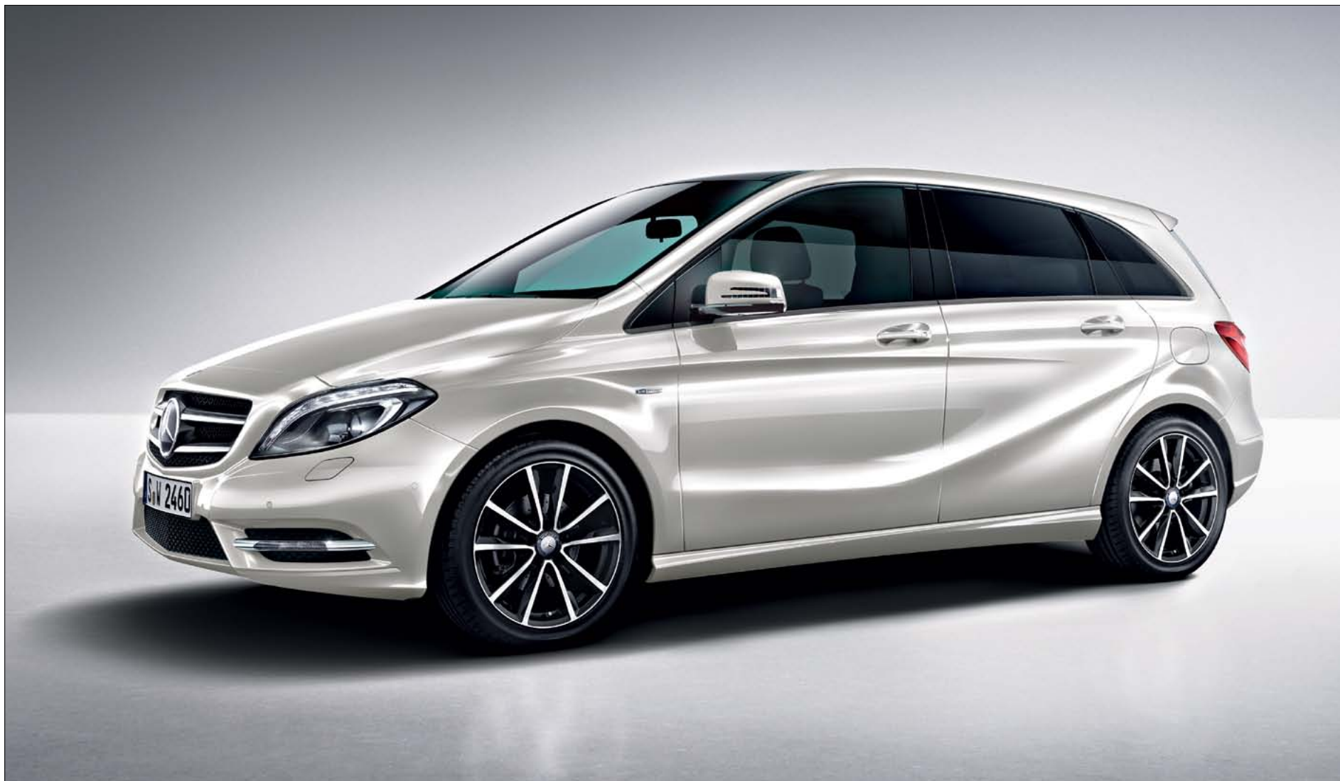
The B-Class Sport is fitted with lowered suspension, 18" bi-colour alloy wheels, drilled front brake discs and optional panoramic sliding sunroof
