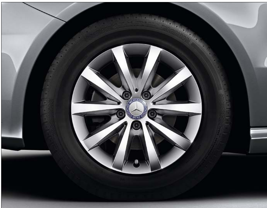
Standard on B-Class SE: 16" 10-spoke alloy wheels, tyre size 205/55 R 16 (code 55R)
