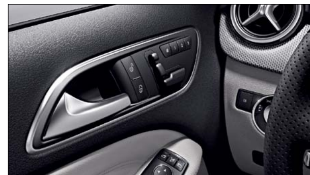
The Memory Package with full electric adjustment stores up to three individual seating positions
