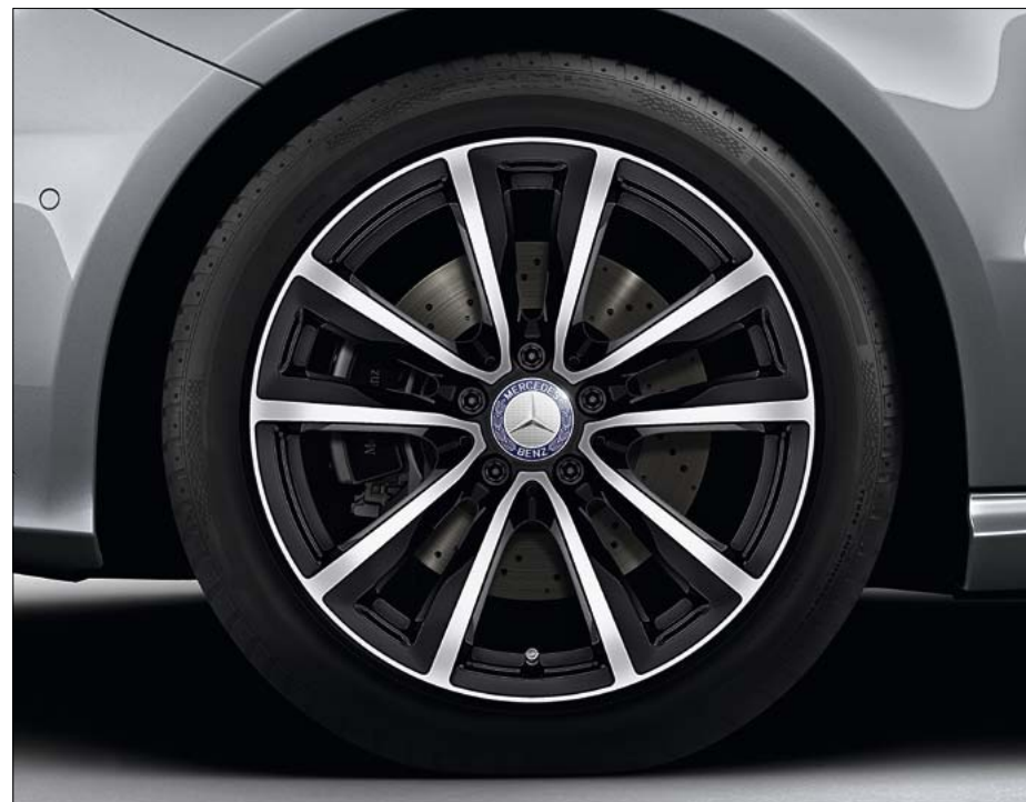
Standard on B-Class Sport: 18" bi-colour alloy wheels, tyre size 225/40 R 18 (code 01R)
