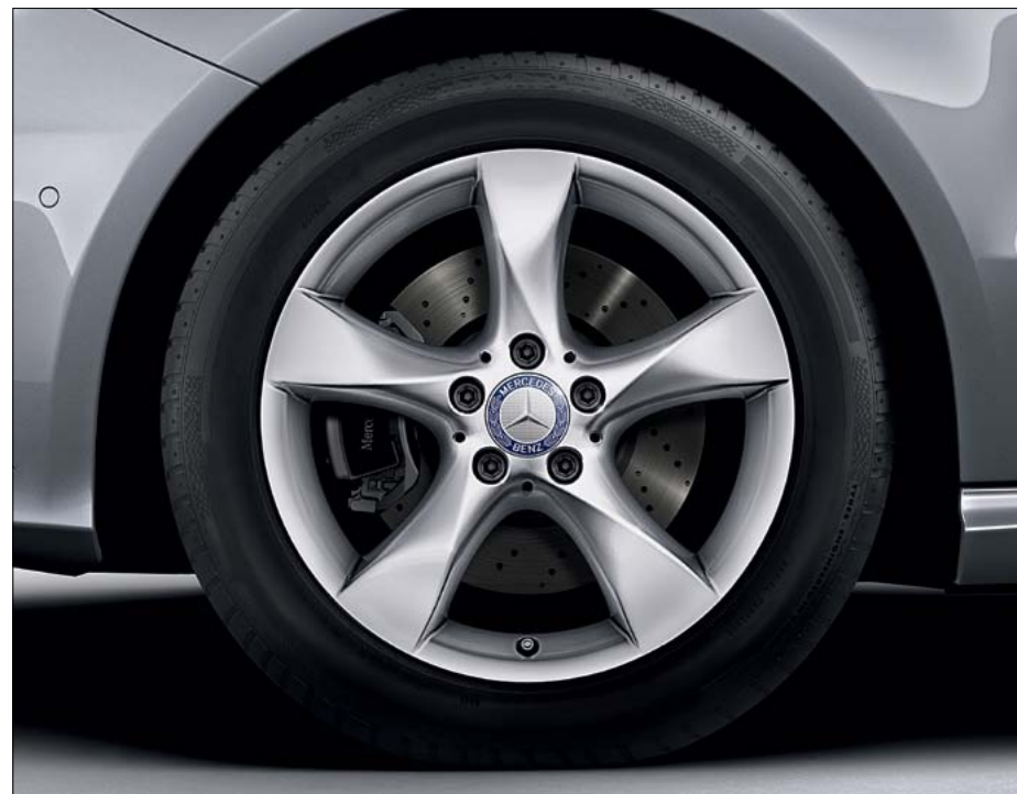
Optional for B-Class Sport at no extra cost: 17" 5-spoke alloy wheels, tyre size 225/45 R 17 (code R24)
