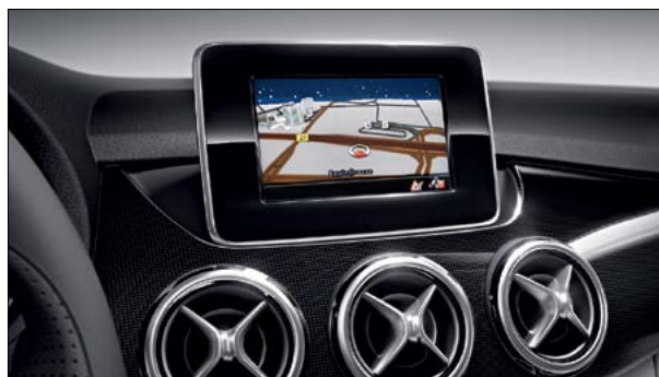
The Becker® Map Pilot system shows vital information both via the Audio 20 CD/radio display, and the multi-function colour display
