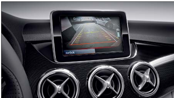
The central COMAND Online display shows the area behind the car during a parking manoeuvre
