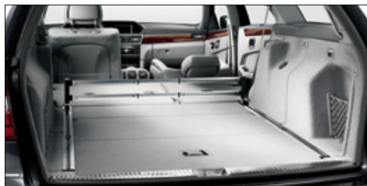
The Easy-Pack folding floor opens to give access to the compartment beneath (shown with optional Easy-Pack load-securing kit)
