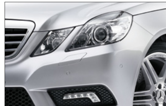
Intelligent Light System with bi-xenon headlamps and LED daytime running lights (standard on Avantgarde and Sport)
