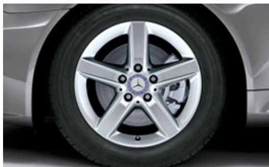
5-spoke light-alloy wheel with 205/55 R 16 tyres at the front and 225/50 R 16 at the rear (standard for SLK 300, optional for SLK 200 KOMPRESSION)
