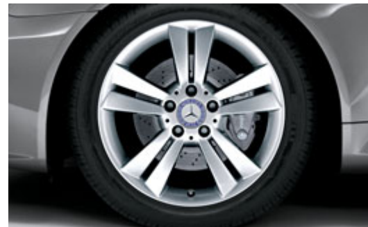
5-twin-spoke light-alloy wheel with 225/45 R 17 tyres at the front and 245/40 R 17 at the rear (standard for SLK 350, optional for SLK 200 KOMPRESSION and SLK 300)
