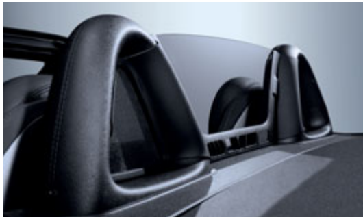
The perspex draught-stop reduces airflow turbulence
