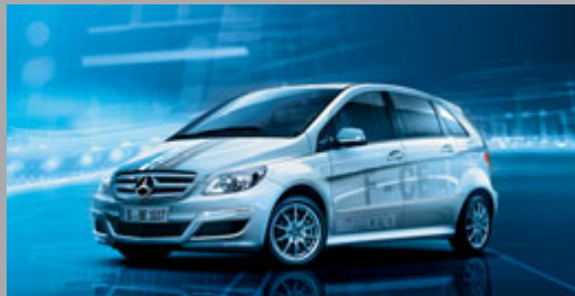
The B-Class F-CELL , with its locally emission-free electric drive system, receives its energy from a fuel cell
