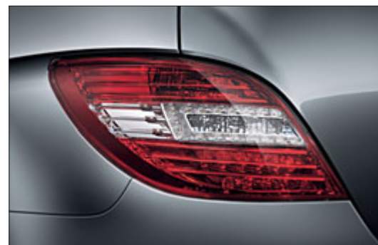
Tail light featuring LED and fibre-optic cable technology
