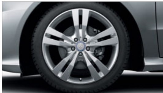
5-twin-spoke light-alloy wheel with 265/45 R 20 tyres (Exterior Sports package, Code R33)
