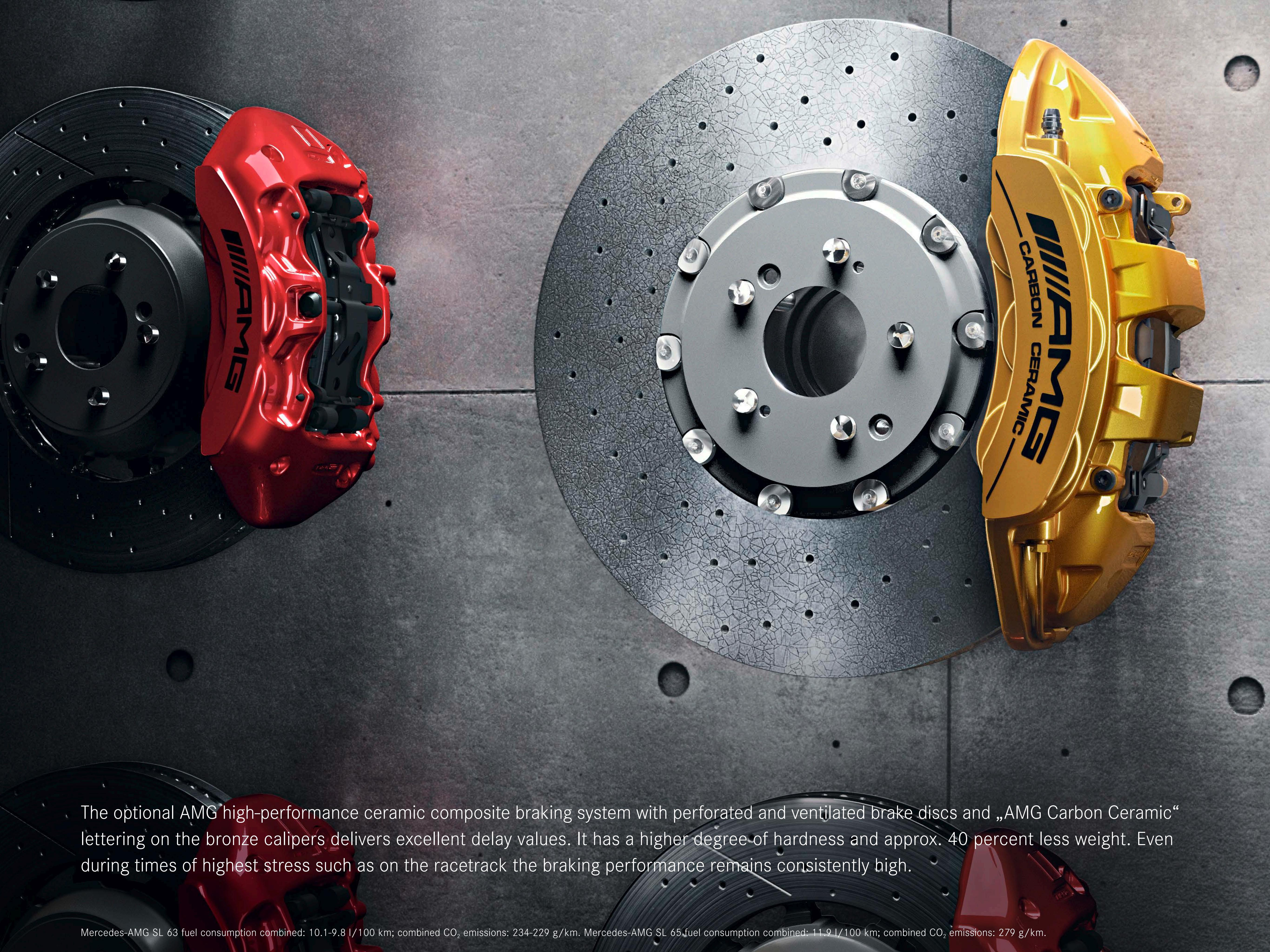
The optional AMG high-performance ceramic composite braking system with perforated and ventilated brake discs and „AMG Carbon Ceramic“ lettering on the bronze calipers delivers excellent delay values. It has a higher degree of hardness and approx. 40 percent less weight. Even during times of highest stress such as on the racetrack the braking performance remains consistently high.
