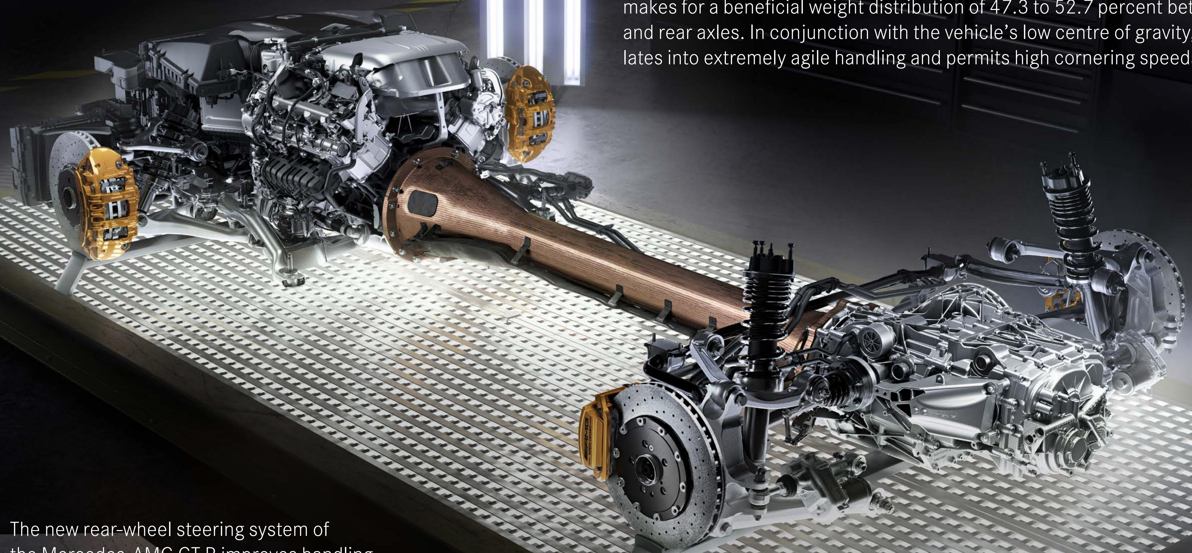
The new rear-wheel steering system of the Mercedes-AMG GT R improves handling safety, while also managing to combine this with comfort, agility and performance. How does it do it? At higher speeds, the rear wheels steer in the same direction as the front wheels, so improving driving stability. At speeds of up to 100 km/h the rear wheels turn in the opposite direction to the front wheels, resulting in improved agility, for example when making a turn or changing direction.
