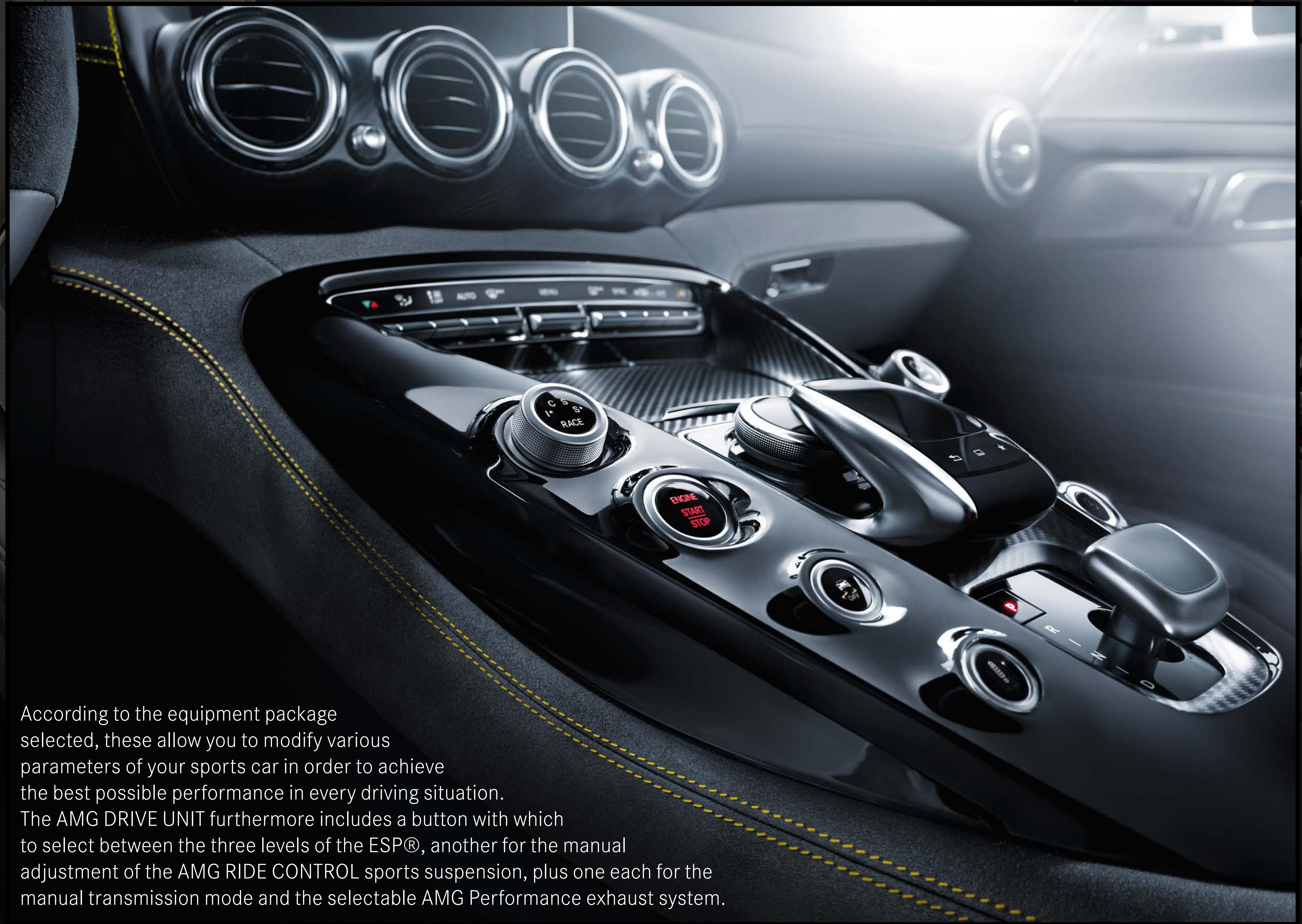
According to the equipment package selected, these allow you to modify various parameters of your sports car in order to achieve the best possible performance in every driving situation. The AMG DRIVE UNIT furthermore includes a button with which to select between the three levels of the ESP®, another for the manual adjustment of the AMG RIDE CONTROL sports suspension, plus one each for the manual transmission mode and the selectable AMG Performance exhaust system.
