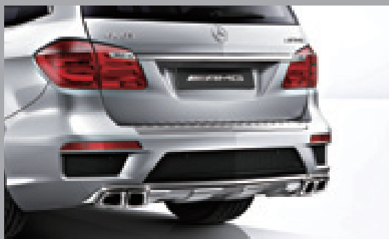
AMG sports exhaust system, tail lights featuring LED fibre optic technology
