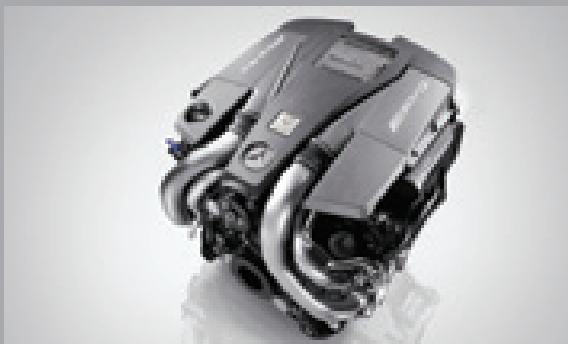
AMG 5.5-litre V8 biturbo engine
