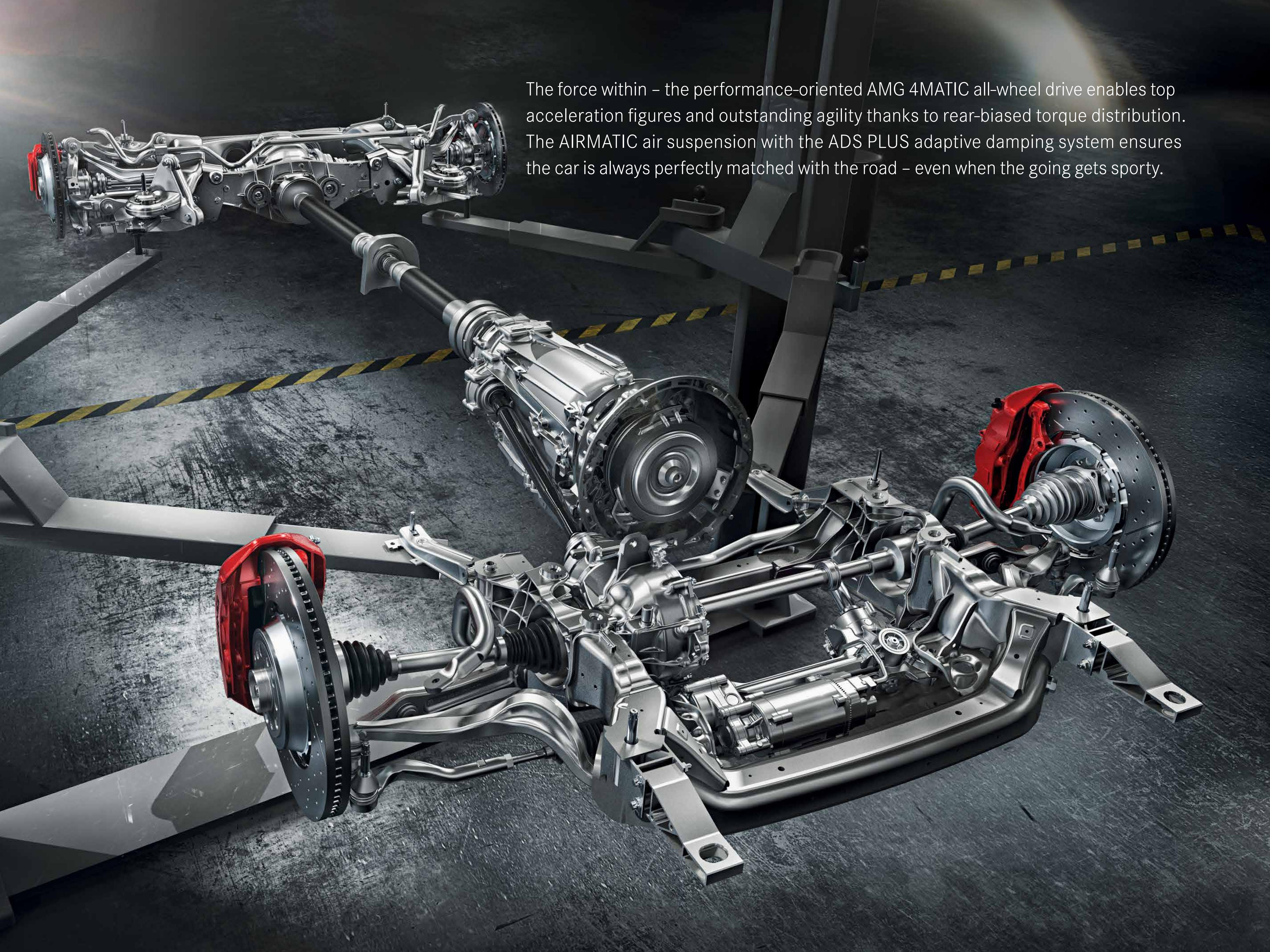
The force within – the performance-oriented AMG 4MATIC all-wheel drive enables top acceleration figures and outstanding agility thanks to rear-biased torque distribution. The AIRMATIC air suspension with the ADS PLUS adaptive damping system ensures the car is always perfectly matched with the road – even when the going gets sporty.
