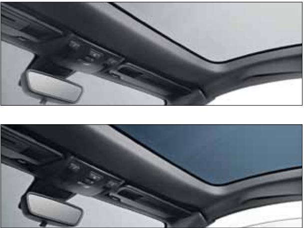
MAGIC SKY CONTROL enables adjustment of the optional panoramic vario-roof's transparency.
