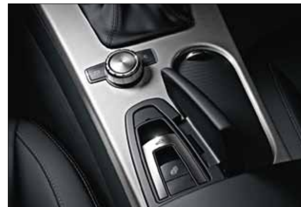
Roof control unit and Controller.
