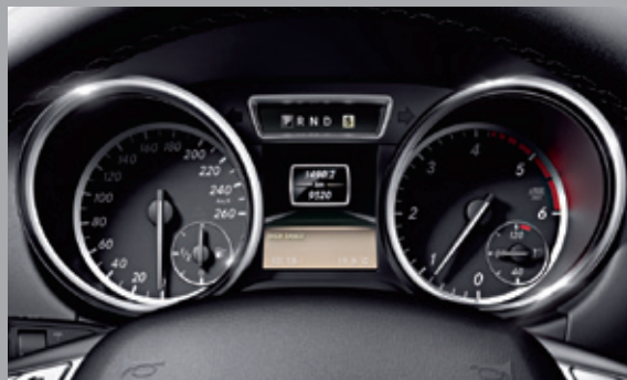
Instrument cluster with 11.4 cm (4.5-inch) TFT display
