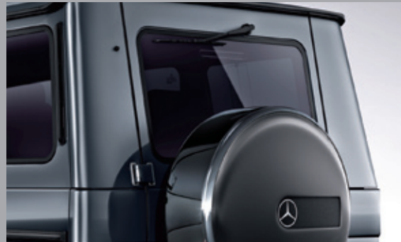
Heat-insulating, dark-tinted glass for rear side windows and rear window
