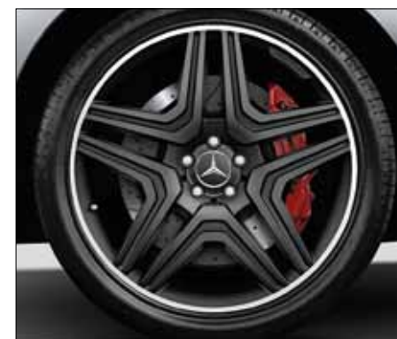
AMG 5-twin-spoke light-alloy wheels with 295/35 R 21 tyres, painted matt black with high-sheen finish, with high-sheen rim flange (optional for ML 63 AMG, Code 685).
