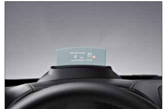
The head-up display shows all the important driving information at a glance.
