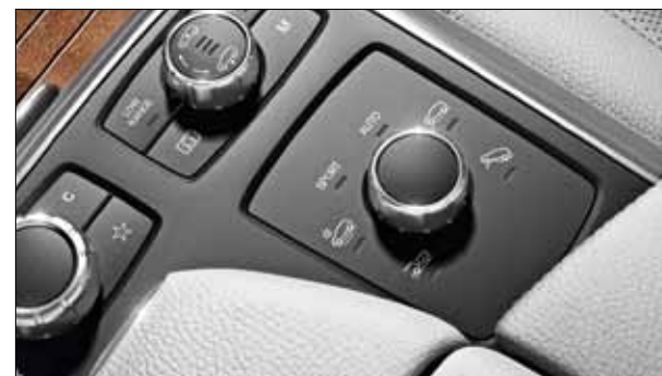
A rotary switch in the centre console is used to set the current driving mode.
