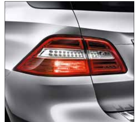
Tail lights featuring LED fibre-optic technology.
