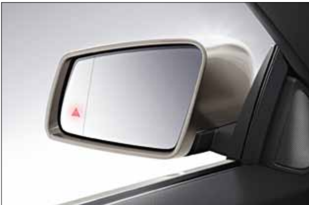
Lane Keeping Assist and Blind Spot Assist can warn the driver in potentially dangerous situations, for instance when changing lanes.
