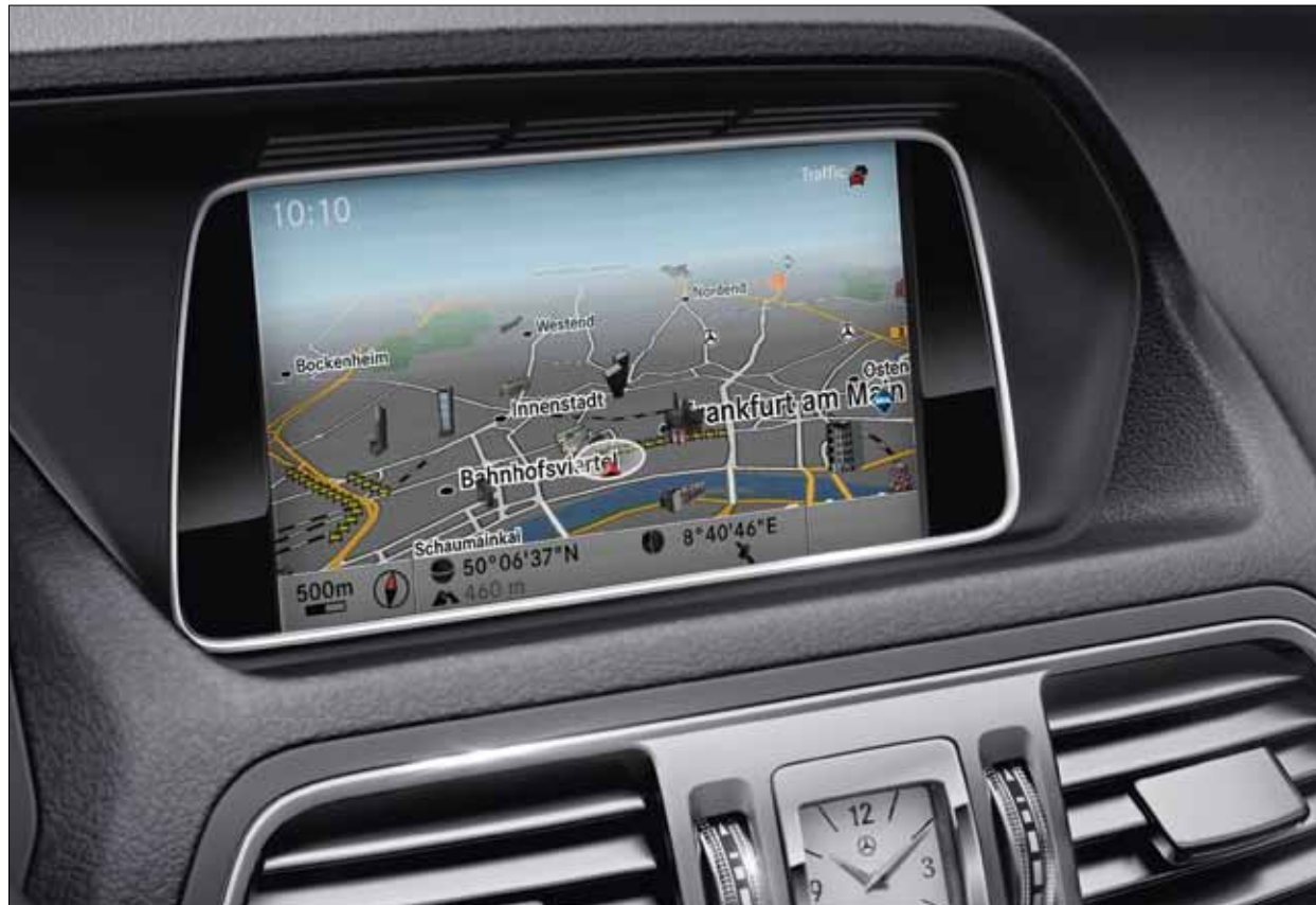
The COMAND Online multimedia system has a flatframe look and a high-resolution 17.8 cm display with TFT technology.
