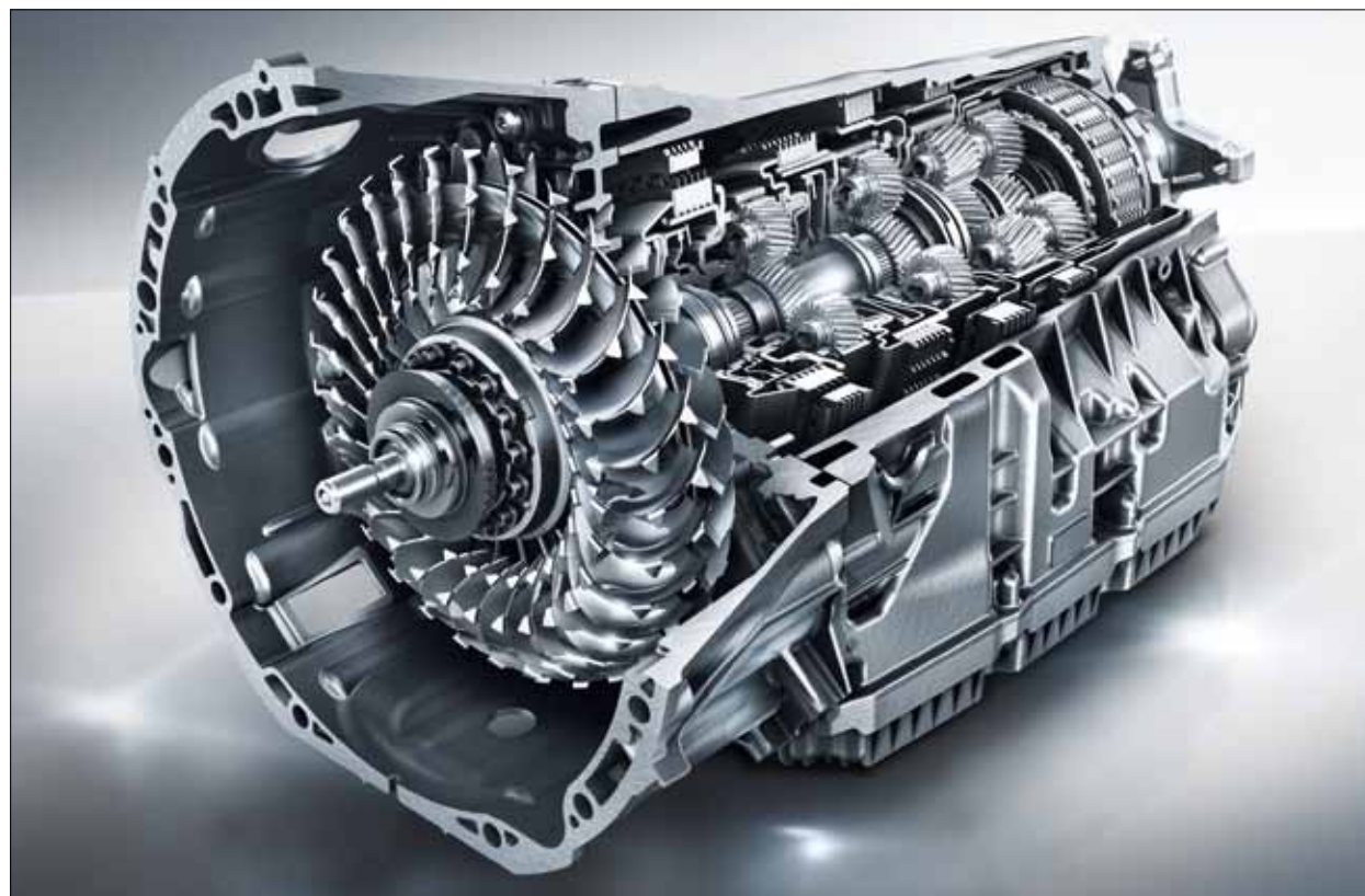
9G-TRONIC: the world's first nine-stage automatic transmission impresses with faster and even more finely graduated gear changes.
