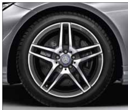
AMG 5-twin-spoke light-alloy wheels, painted titanium grey with a high-sheen finish, with 235/40 R 18 front tyres and 255/35 R 18 rear tyres (code 660, part of AMG Sports package).
