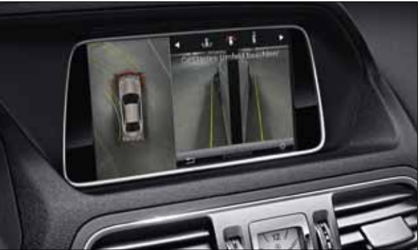
During parking, the COMAND Online central display shows the area around the car.
