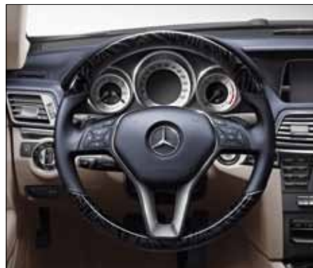
Wood/leather multifunction steering wheel with steering-wheel gearshift paddles.
