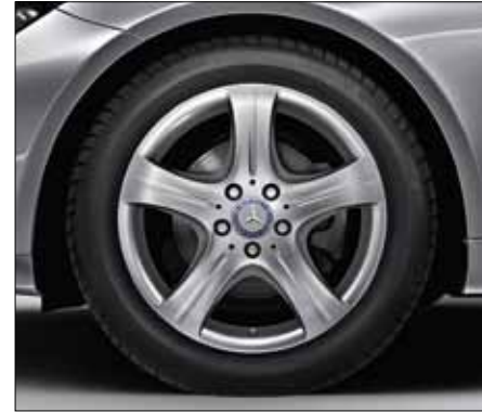
5-spoke light-alloy wheels with 235/45 R 17 front tyres and 255/40 R 17 rear tyres (optional for 4- and 6-cylinder models, code R22).
