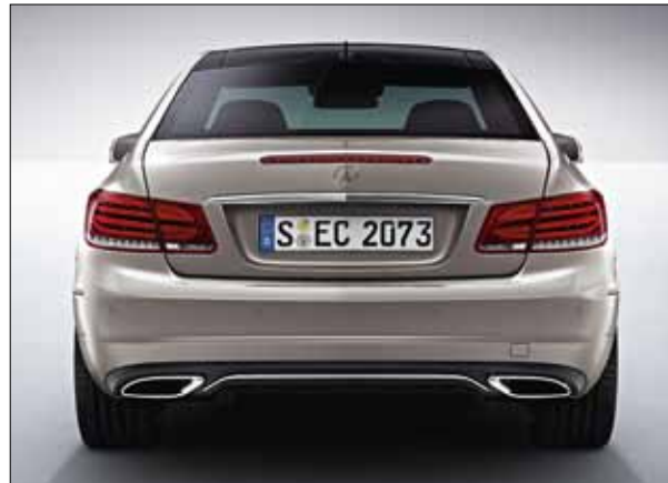
The Exterior Sports package with a two-pipe exhaust system featuring trapezoidal tailpipe trims in polished stainless steel integrated into the bumper.
