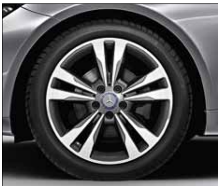
5-twin-spoke light-alloy wheels with 235/40 R 18 front tyres and 255/35 R 18 rear tyres (optional, code 22R).
