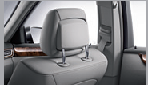
Crash-responsive NECK-PRO head restraints in the front
