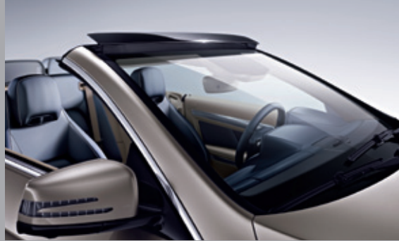
AIRCAP with electrical air deflector module
