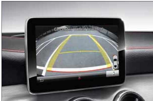
The reversing camera supports the driver when backing into a parking space. It is available in conjunction with Audio 20 USB and COMAND Online.
