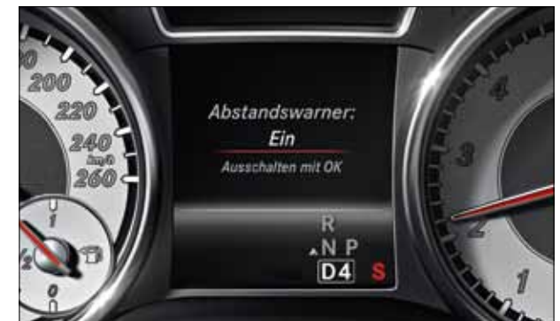
COLLISION PREVENTION ASSIST PLUS can give the driver visible and audible warnings if the safety margin is too short.
