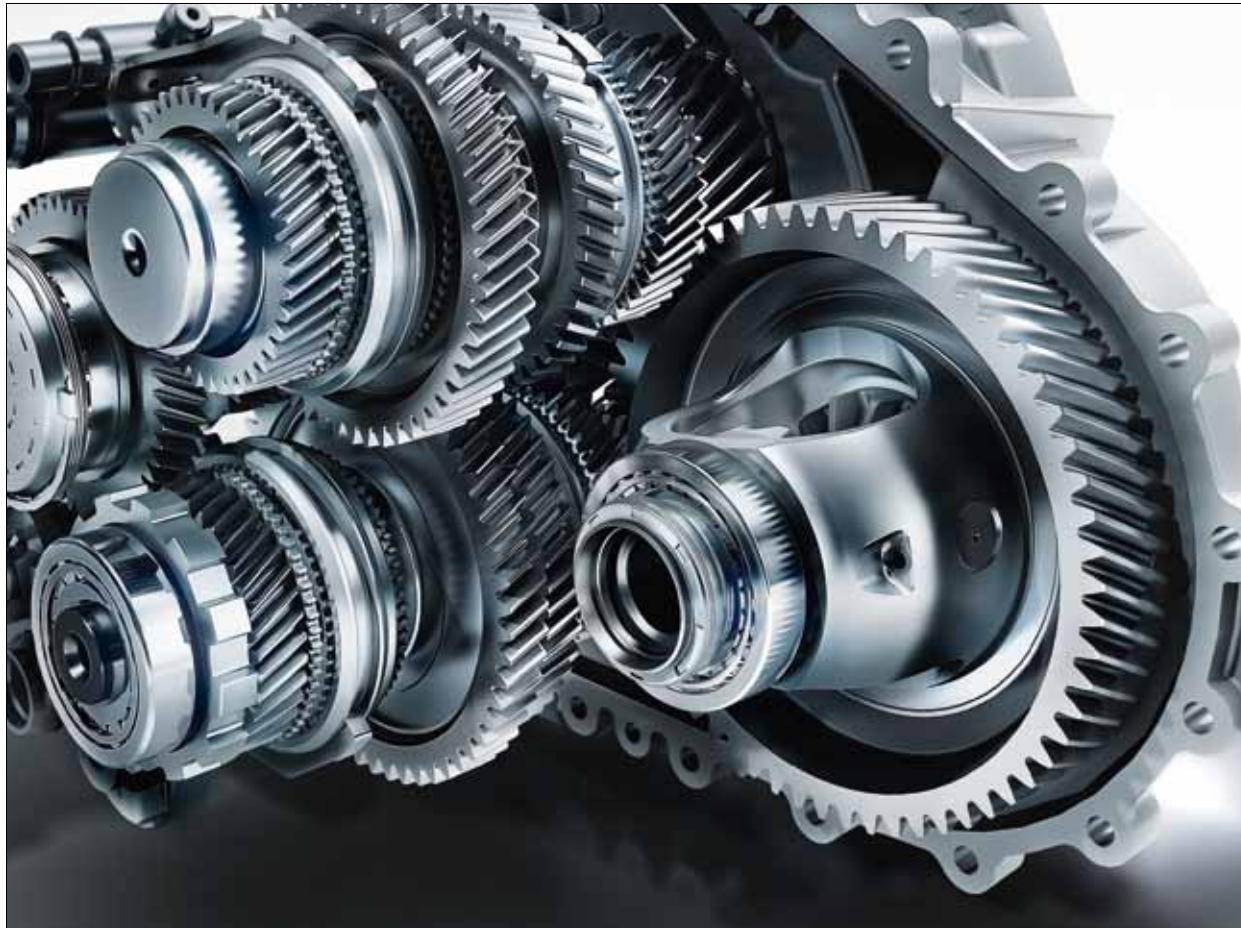
The seven-speed dual clutch transmission 7G-DCT enables gear shifting without any interruption in tractive power.
