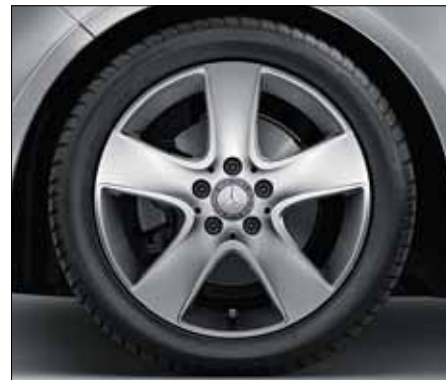
5-spoke light-alloy wheels with 225/45 R 17 tyres, painted titanium silver (option, Code R24).
