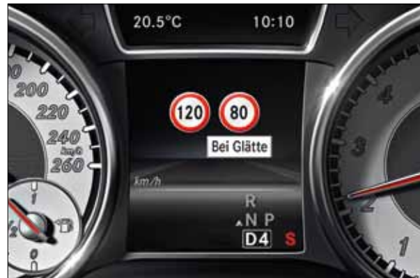
The information from Traffic Sign Assist is shown both in the instrument cluster and on the COMAND Online central display.
