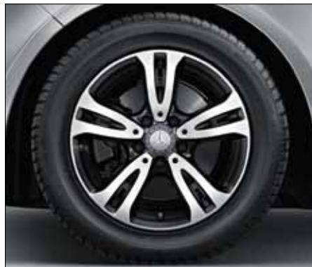
5-twin-spoke light-alloy wheels with 205/55 R 16 tyres, painted matt black with a high-sheen finish (option, Code R78).
