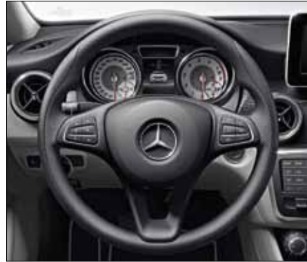
12-button three-spoke multifunction steering wheel.
