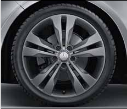
5-twin-spoke light-alloy wheels with 225/40 R 18 tyres, painted himalayas grey (option, standard for Urban, Code 66R).
