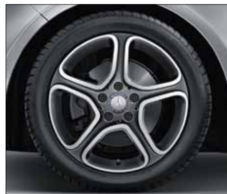
5-spoke light-alloy wheels with 225/45 R 17 tyres, painted tremolite grey with a high-sheen finish (option, Code 02R).
