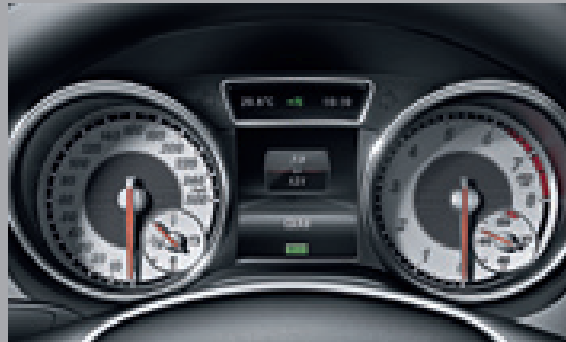
Instrument cluster in 2-tube look with colour TFT multifunction display
