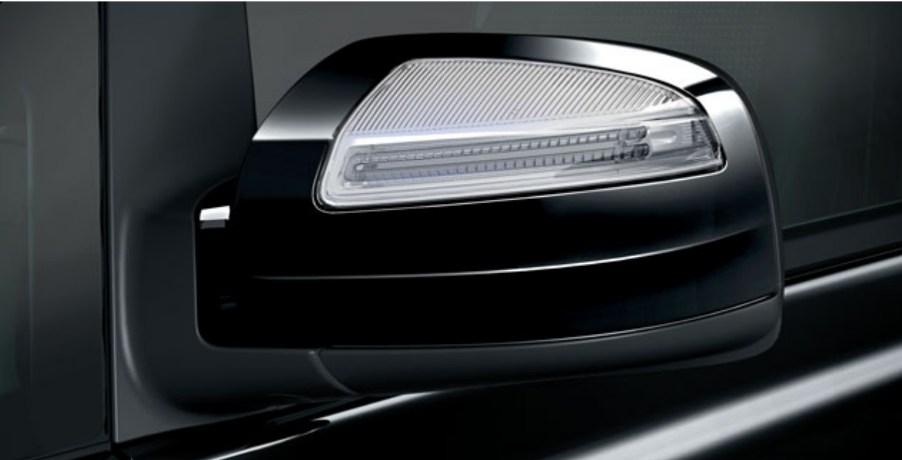
Exterior mirror with aspherically curved glass and integrated turn indicator lamp, electrically adjustable.
