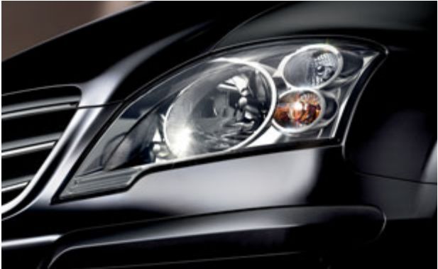
Reflective headlamps with integral front fog lamps and daytime driving lights (not available for the Viano AMBIENTE or Viano AVANTGARDE).
