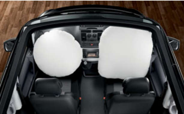
Driver and front-passenger airbags (picture shows activated airbags at maximum deployment for illustrative purposes only).
