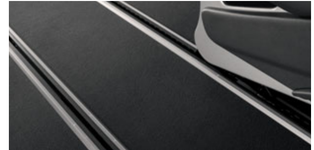
Seat rail system for variable configuration of the interior.
