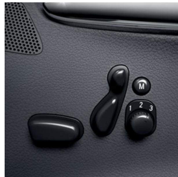
Driver's and front passenger seats electrically adjustable with 3 memory settings.
