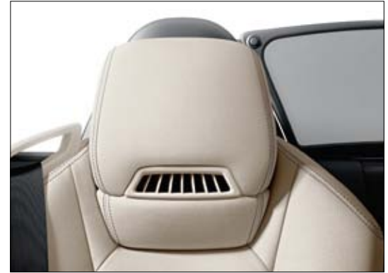
Aircarft neck-level heating vents in head restraints
