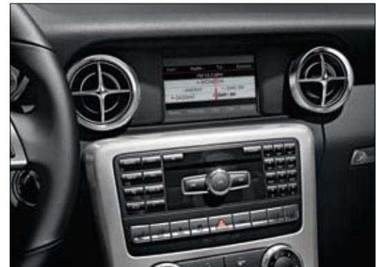
Audio 20 radio with integrated 6-disc CD changer
