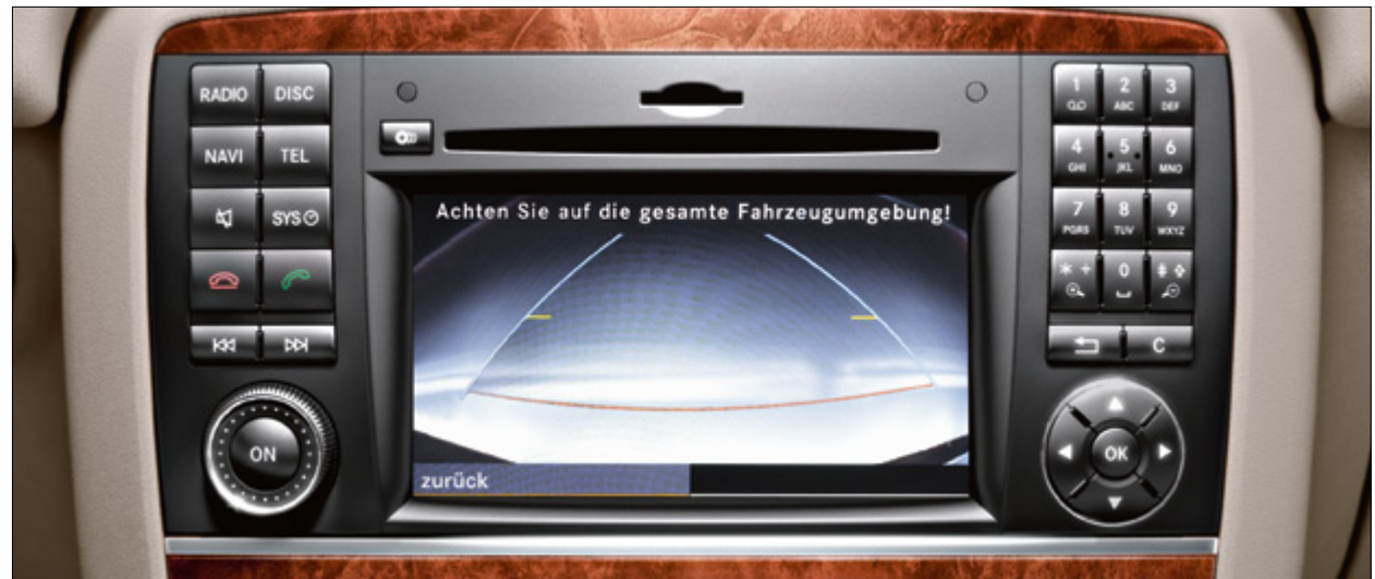
The reversing camera captures the area immediately behind the car
