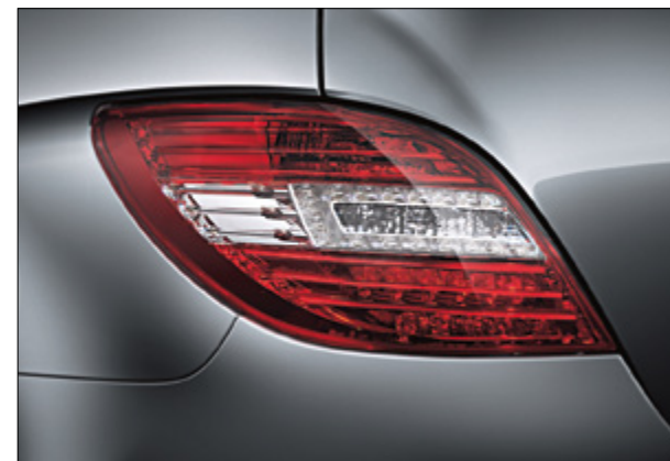
Tail lights featuring LEDs and fibre-optic technology
