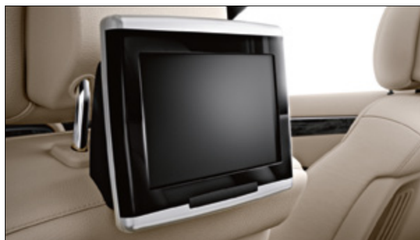
The displays for the rear seat entertainment system are mounted on the backs of the front seat head restraints
