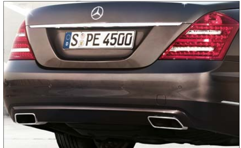
Rear bumper with integrated tailpipes and LED rear tail lights
