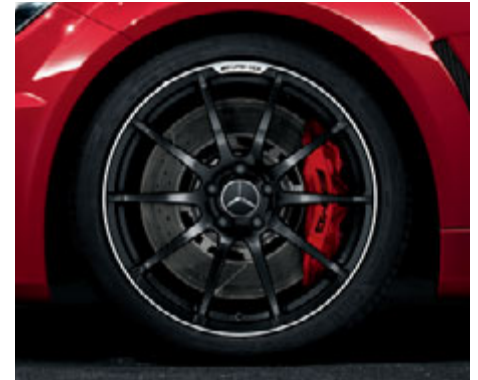
10-spoke AMG forged wheels with 255/35 R 19 front and 285/30 R 19 rear tyres, painted matt black, rim flange with high-sheen finish (optional)
