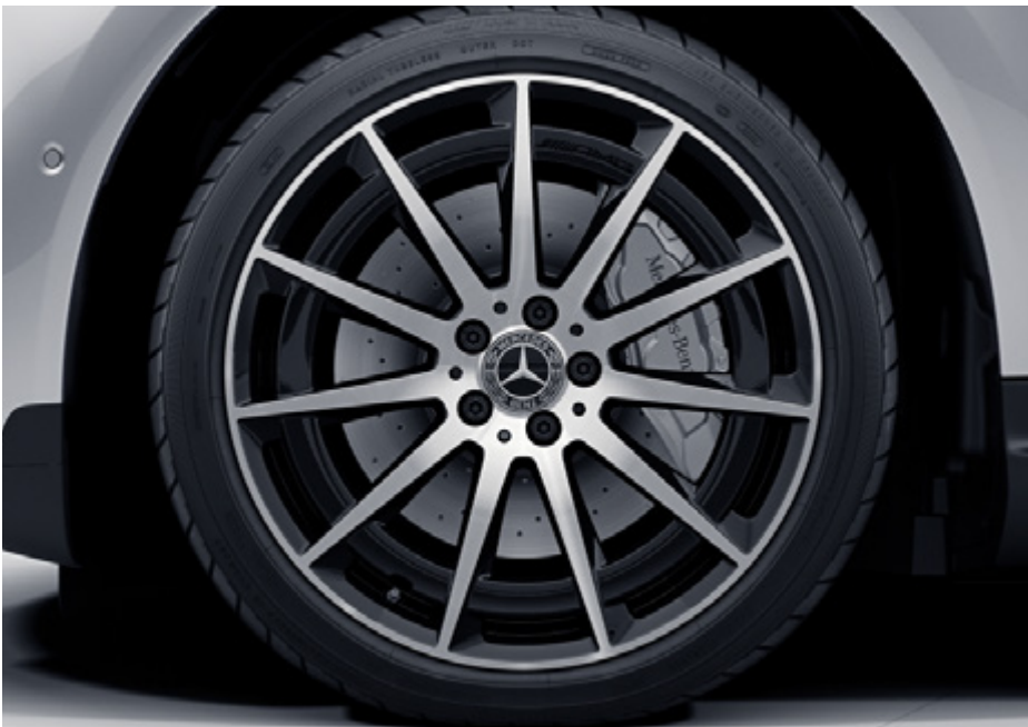
RRR 20" alloy wheels (4) – multi-spoke aero design, painted black with a high-shine finish front: 235/55 R 20 tyres; rear 255/45 R 20 tyres
