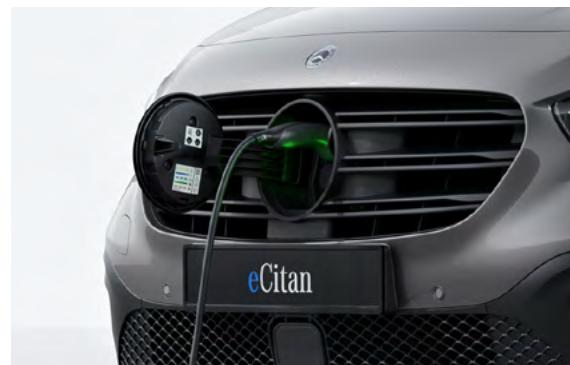
CCS rapid charging port, 75kW max. capacity.
