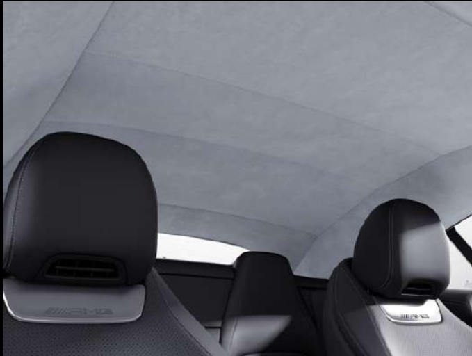
69U Roof liner in DINAMICA microfibre – neva grey
