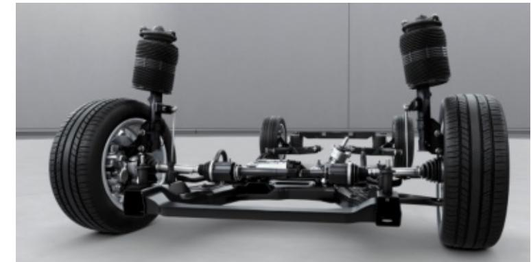
No matter if you are on the motorway or a track with ruts: the **AIRMATIC** air suspension can adjust the suspension to suit the road surface. Damping can be regulated for each individual wheel automatically – to suit the current driving situation and the state of the road.
