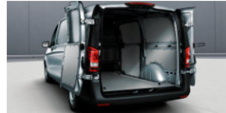
The **double-wing rear doors** can be opened back to the sidewalls and secured, making loading and unloading easier.
