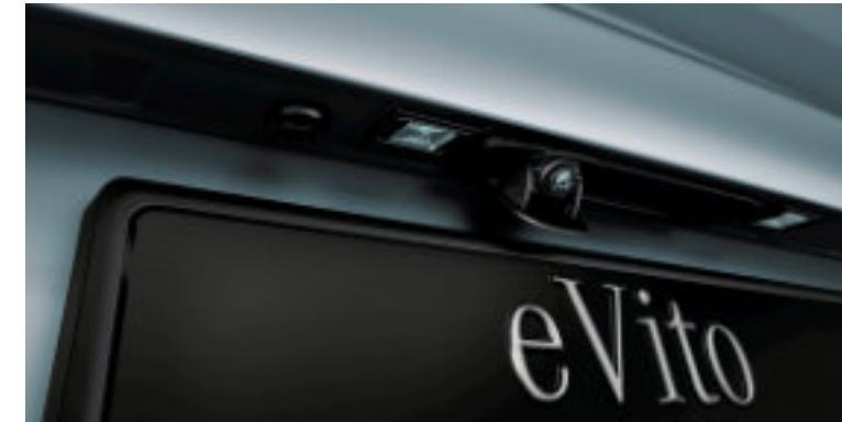
The **reversing camera** assists you when parking and manoeuvring: it displays the area behind the vehicle, which you cannot see directly. As a result, damage caused when parking and manoeuvring can be avoided.
