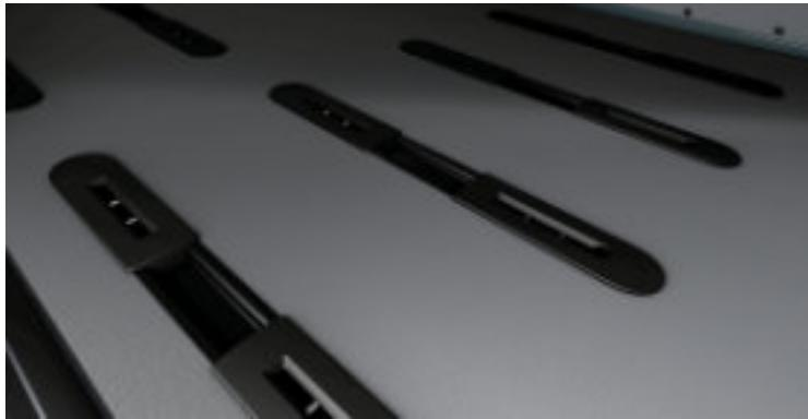
The **load anchoring system** allows proper and flexible securing of the load. Objects can be secured on the 2 anchoring rails on the load compartment floor with the help of the optional lashing eyelets and securing straps.
