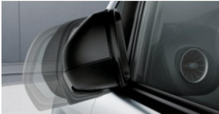
The **Vito Mirror Package** uses automatically dimming mirrors and electrically folding outside mirrors to increase the driving comfort and driving safety.
